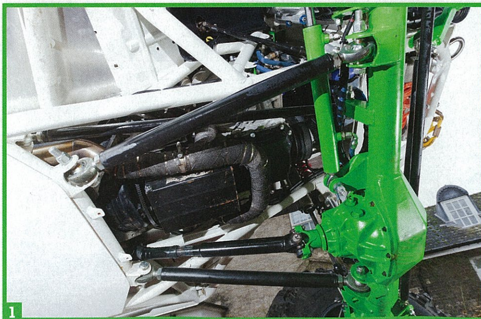
Seen from underneath, the complexity of the vehicle's T45 spaceframe chassis becomes apparent. The integral skid-plate helps it slide over rocks and extreme crests. What this view shows particularly well, though, is the geometry of the linkages used on both axes; three-link up front, with an offset third link between the two main radius arms, and four at the rear. Inside both axes is a True High 9 diff containing an ARB RD99 Air-Locker, as well as a set of 300M CV joints and halfshafts
